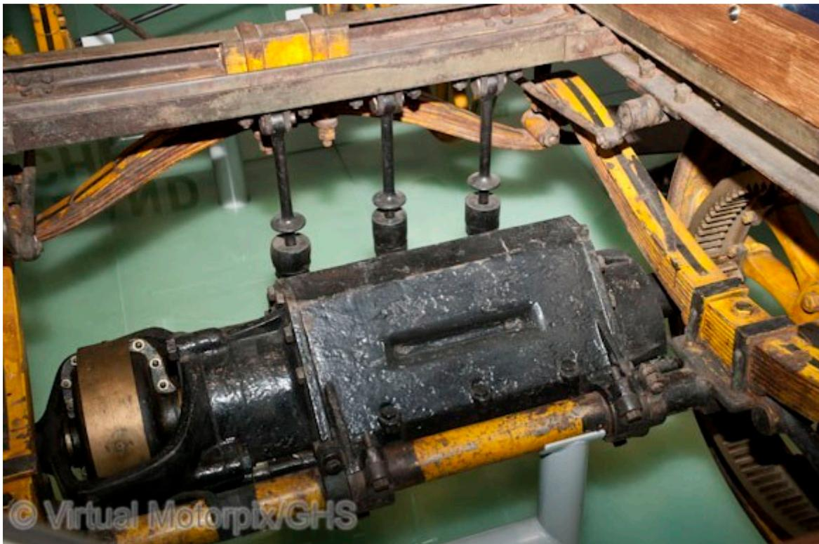
The P1's 'octagon' electric motor sits between the front and back wheels
