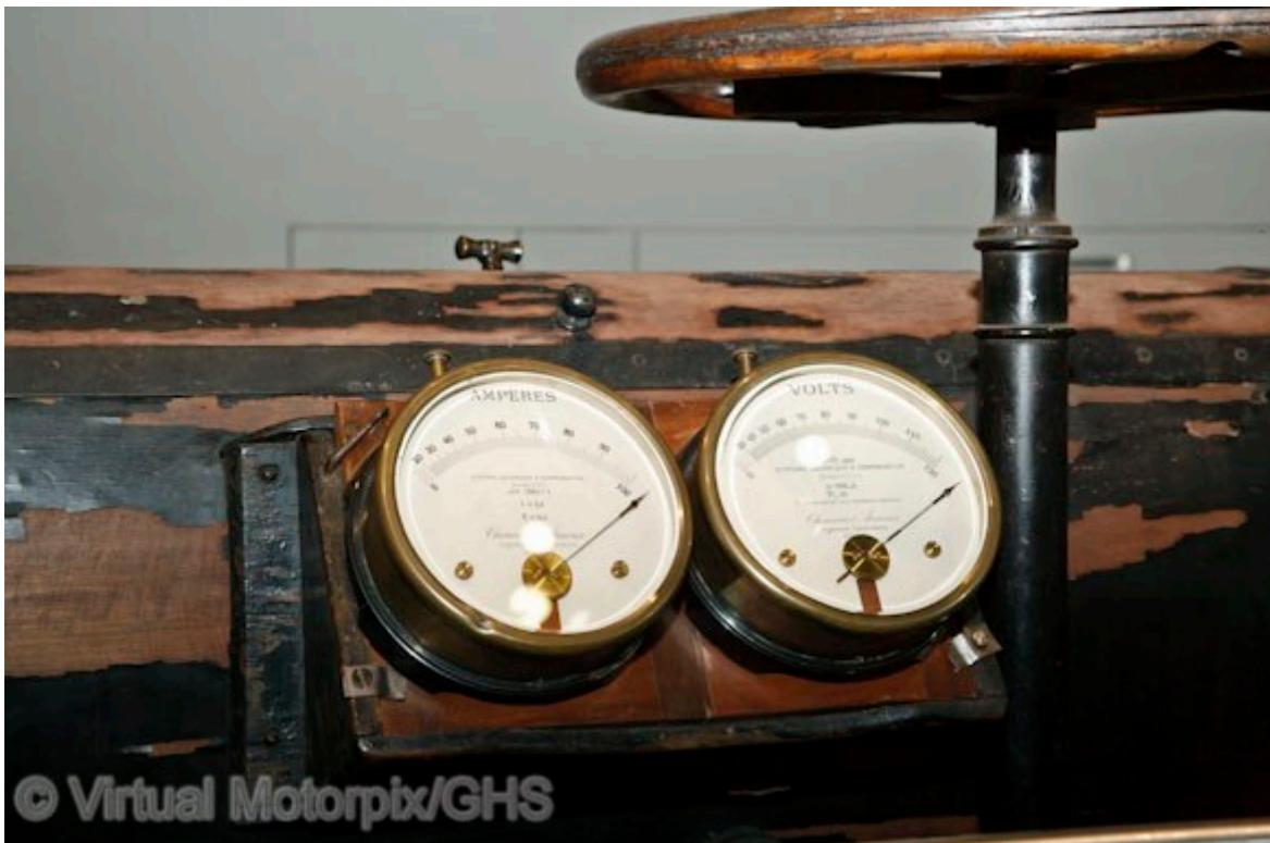
Amps and Volt meters in the P1 were the speedo and rev counter of the day
