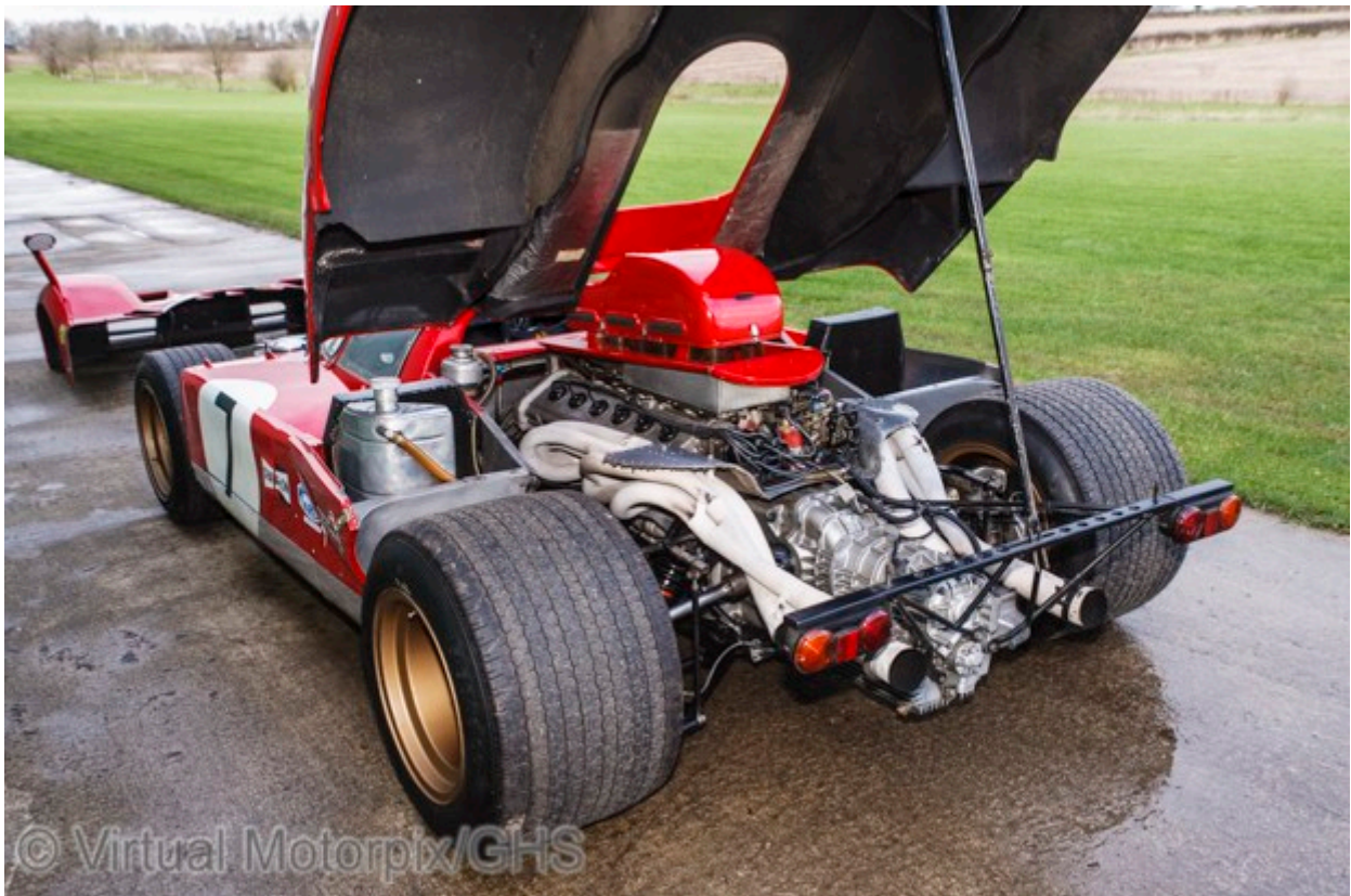
Showing the business end of the 1970 5 litre V12 Ferrari 512 S (chassis 1026)
